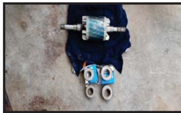
Photo No.2 Change bearing.
